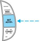
• Accelerate with your accelerator pedal. When the desired vehicle speed is reached, press and release SET/SET ACC/SET ACCEL.
